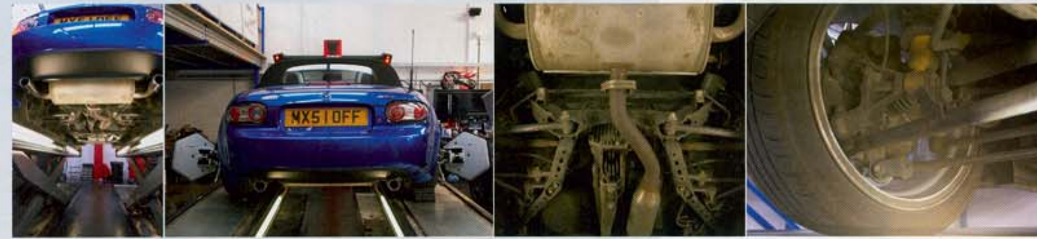
Below: David Bell's 2.0i Sport has lost its lofty stance thanks to Mazda-approved Eibach sport springs. Feels a lot better too. However, session on chassis rig at WRC Technologies (above) reveals alignment is outside recommended tolerances, suggesting dealer that fitted springs didn't check the geometry afterwards. Above right: MX-5's set-up is very tweakable
